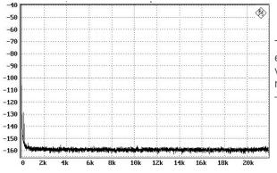
The results are limited by the capabilities of the measuring equipment and noise floor lays at -160dB or even lower. There are visible peaks at 50Hz and 100Hz which are caused by limits of the measuring instruments. However, they are at a level of -130dB and -140dB.
