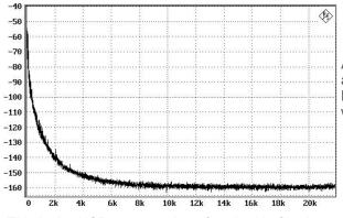
After applying passive RF interference filtering the results are already remarkable. Noise on 1kHz drops to -125dB, at 10kHz Noise comes even close to -160dB. But they improve even further when applying an active filter after the passive filtering.
