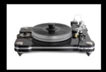
The 1.75"-thick platter is comprised of clear or black acrylic and incorporates an inverted bearing similar to that used in the HR-X. The bearing shaft is 60 Rockwell hardness, ground and polished, and the platter rotates on a Teflon/Delrin composit thrust plate for ultra low noise.
