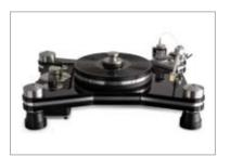
The HR-X features a triple laminated chassis (Acrylic-Aluminum-Acrylic), integral air suspension (which rejects up to 98% of acoustic feedback) and an inverted main bearing incorporating a hardened steel ball running on a Teflon/Delrin composite.
