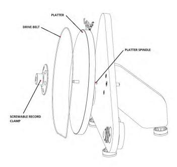
After the placing the record on the platter, it is necessary to tighten the screw-able record clamp (6) onto the platter spindle.
