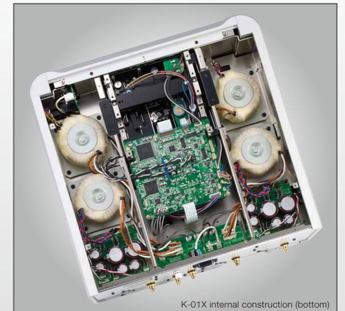
K-01X internal construction (bottom)
